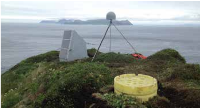
A UNAVCO GPS/GNSS installation on the Aleutian Chain.
